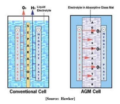
If you replace a sealed maintenance free battery in a GM car with a non-sealed *lead-antimony or lead-antimony/calcium* low maintenance battery, you will need to check the electrolyte levels more often. This is because GM sets their voltage regulators at higher charging voltage, 14.8 volts, to recharge the sealed maintenance free lead-calcium/calcium batteries, like the original AC Delco batteries.
