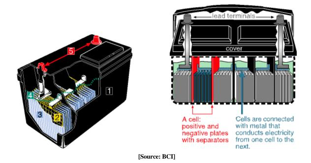
After the "curing" of the plates, they are made up into cells, and the cells are inserted into a high-density tough polypropylene or hard rubber case [#1 in the diagram above]. The cells are connected to the terminals [#5 in the diagram above], and the case is covered and then filled with a dilute sulfuric acid electrolyte [#4 in the diagram above]. The battery is initially charged or "formed" to convert yellow Lead Oxide (*PbO or Litharge*) into Lead Peroxide (*PbO2*),
