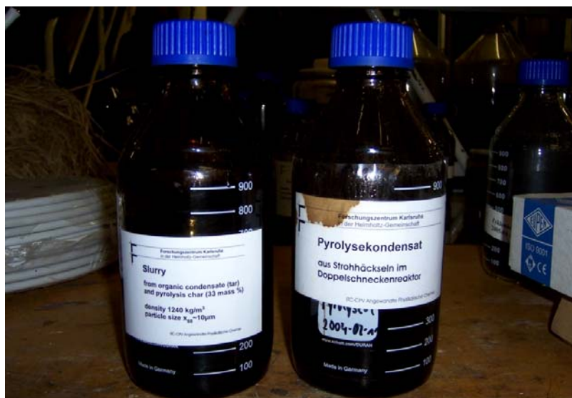
Figure 40: Slurry produced with the bioliq process
