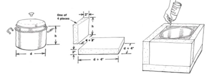
**Figure 1:** Cut and glue together five pieces of two-inch styrofoam pieces, insert well-waxed pot after removing the handles, and fill empty spaces with expanding foam insulation. Note the dimensions of the five foam pieces.
