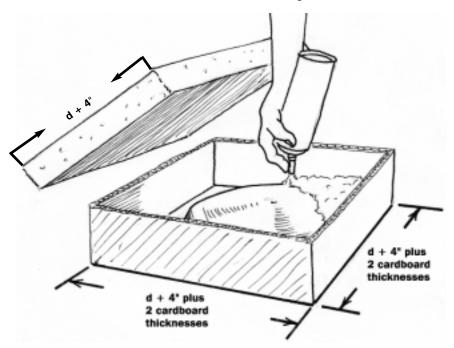
**Figure 2:** Place waxed lid (after removing lid handle) inside waxed cardboard box, cover with expanding foam insulation, then press piece of two-inch thick foam insulation into box, on top of the expanding foam. Note the dimensions.
