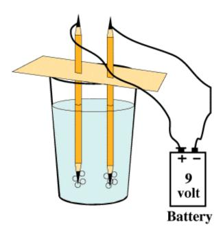
Dissolve about a teaspoon of salt into the warm water and let sit for a while. The salt helps conduct the electricity better in the water.
