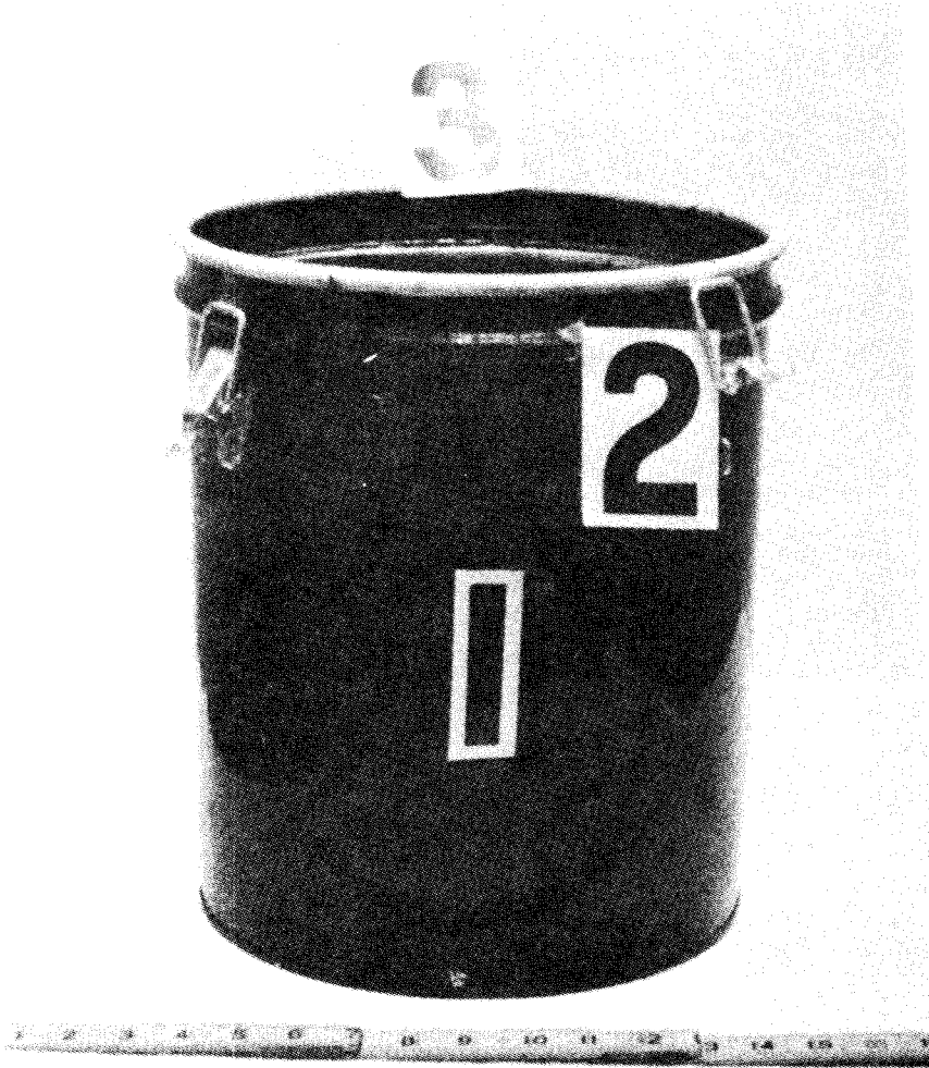
Fig. 2-21. Filter container (#1) showing latches (#2) for lid and hose (#3) around top.
