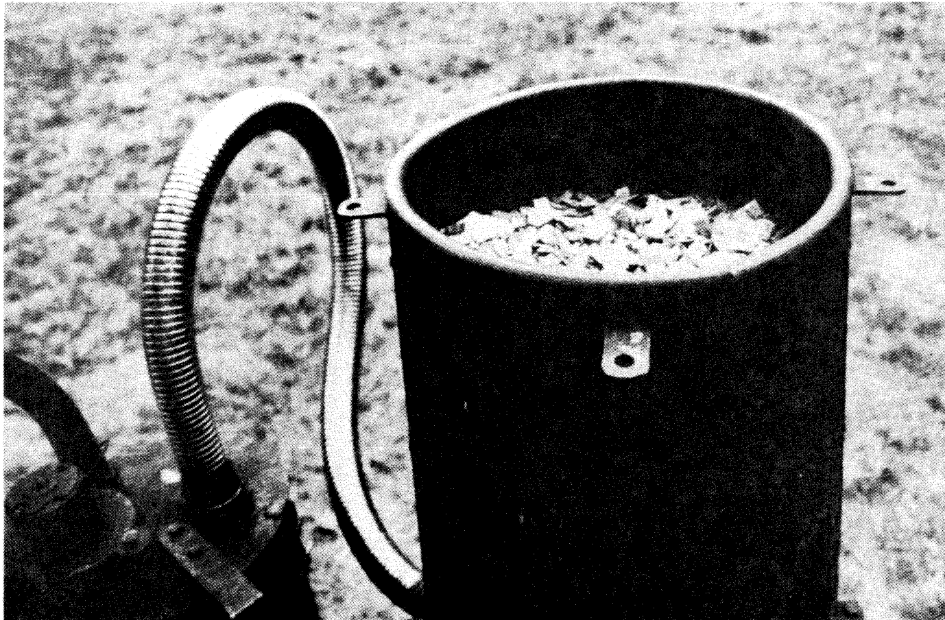
Fig. 3-1. Virtually all varieties of wood chips can be used for fuel. (Minimum size for this 6-in. firetube unit: 3/4 by 3/4 by 1/4 in.; maximum size: 2-in. cubes.)
