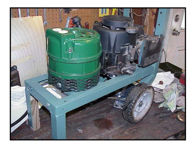
View showing generator slider for belt adjust.
