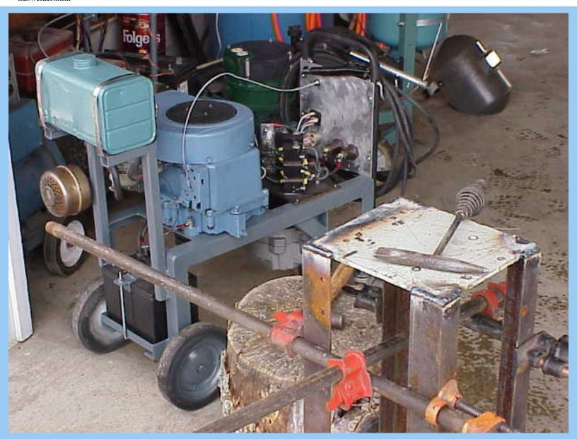
Project of the day: A disc grinder stand with 33" high mounting plate. (Legs are not flared out yet)
