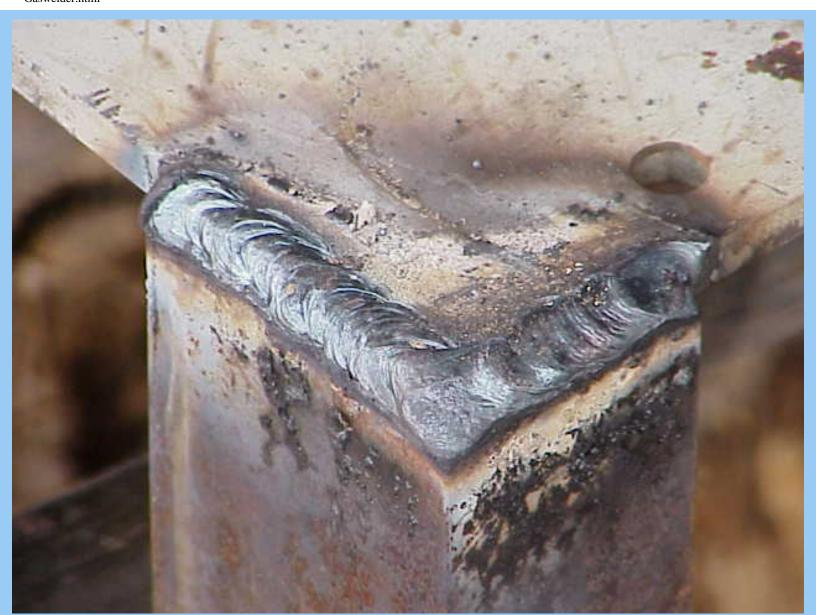
Close up of weld, 1/4" steel plate to 1/8" legs. Welded at about 85 amps, with a 3/32", Lincoln 6013 electrode.
