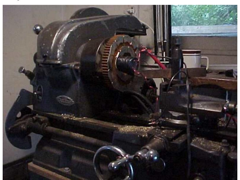
Next step was to turn it on, and test the different taps on the coil, at 3 different speeds. I used a 12 Volt, 5 watt light bulb as a load, and tested the voltage of each tap on the coil, at each speed, with, and without the load. The tests were done at 200, 400, and 600 RPM.
