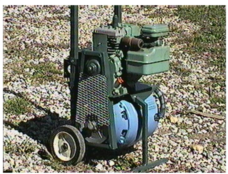
In this view, the belt guard is visible, while the generator is below the engine stand.
