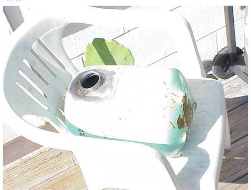
Freon tank converted to a gas tank. The fittings were cut off an old gas can and silver brazed to the tank. Standard 1/4" pipe fittings were used for the outlet pipe. Fuel filter is not in the tank, but in the fuel line.
