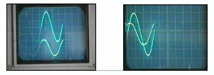
Top Trace: 60 hertz / Bottom Trace: Capacitor phase shift. Overlaid waveforms.
