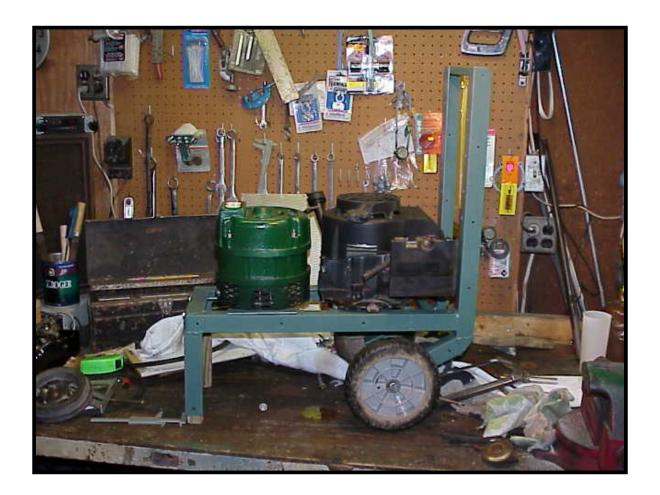
Generator on its new mounting frame with a B&S 5 horsepower Quantum engine.
