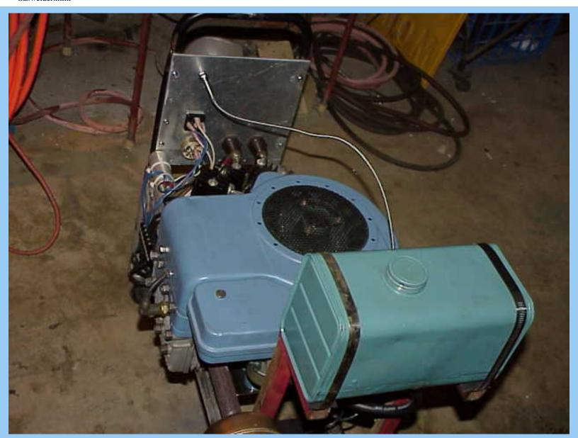
A one gallon gas tank provides a couple of hours of continuous operation.
