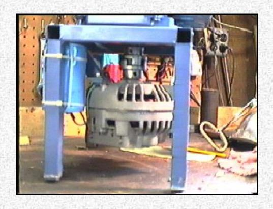
Front view of the alternator. Note the 89000uf filter capacitor (Blue cylinder behind the front left leg) used at the output to filter the output voltage.
