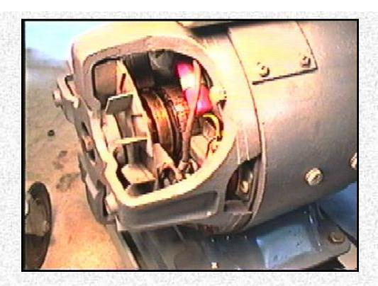
Here are the "innards" of the generator. (Rear shroud removed) Note the AC slip rings (only one is visible), the DC commutator, fan and noise supressor capacitor.
