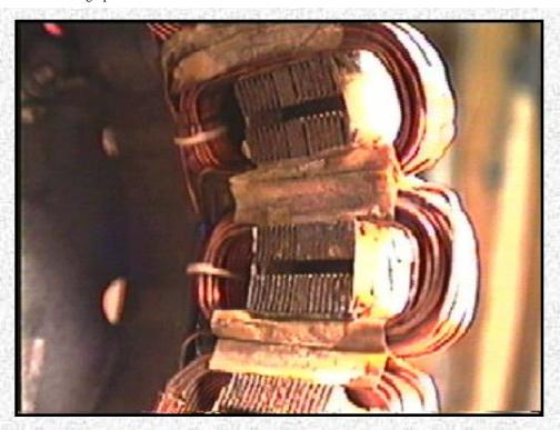
In this close-up shot, notice the two pole faces wound as one and where each third pole has been cut out. A small coil form was made out of plexiglass to wind the coils. I used epoxy glue to hold the coils in place, with fiber tape as an insulator. The coils are about 36 turns of #18 wire, all connected in series.
