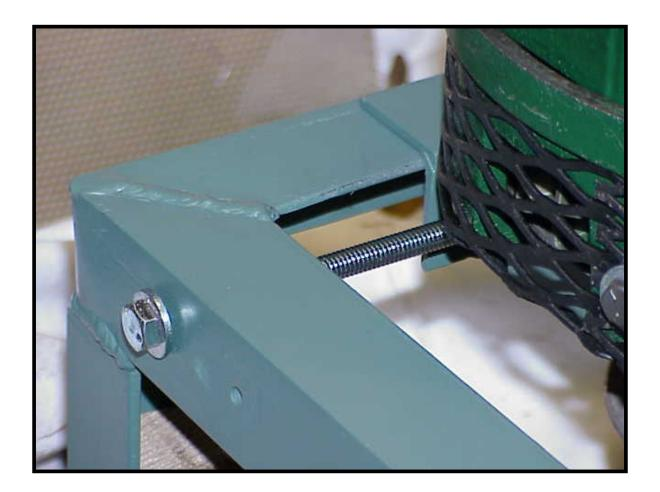
Bolt used to adjust tension on the drive belt by pulling generator slide away from the engine.
