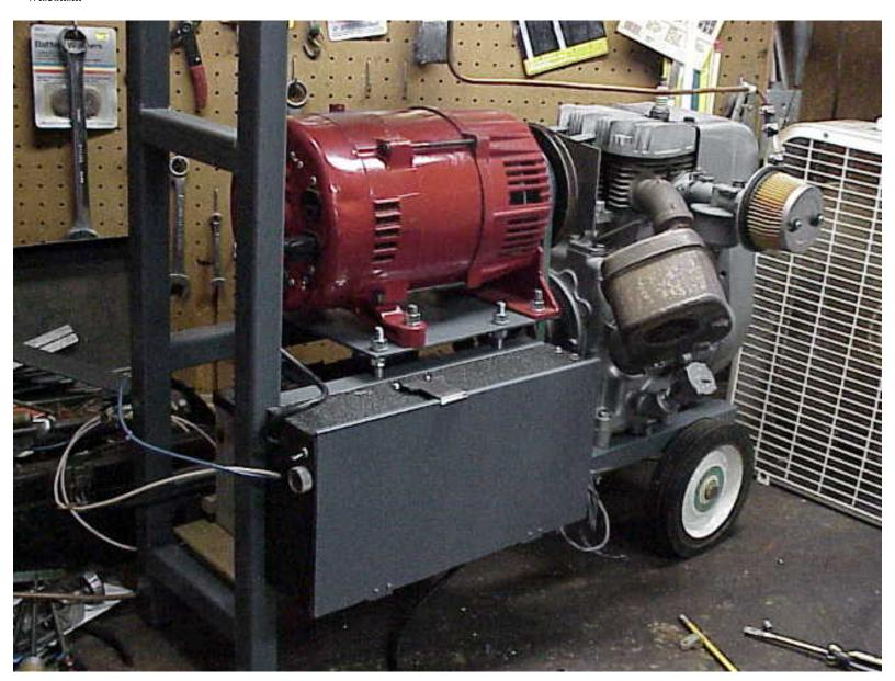
The fun part is attaching the gen and engine to the frame. It's cool when it all comes together! The battery is mounted under the generator and is just visible behind the control box.
