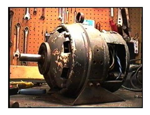
In this generators original configuration, it was driven by a 3 horsepower, single phase, 124/240VAC 60 hz, electric motor. The outputs were 12 VDC at 25 amps and 120 VAC, 400hz, at 10 amperes. The motor and generator were mounted on a steel frame and weighed in at about 150 pounds. Definitely Navy surplus, as one of the grease fittings called for Navy type grease.
