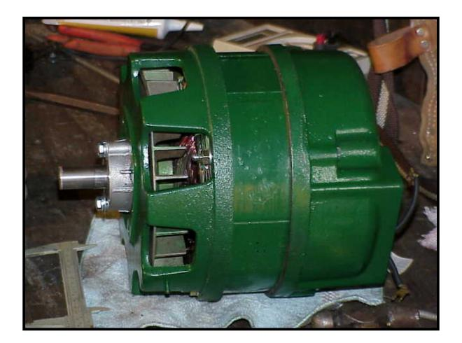
Note outboard bearing housing on front in this picture.
