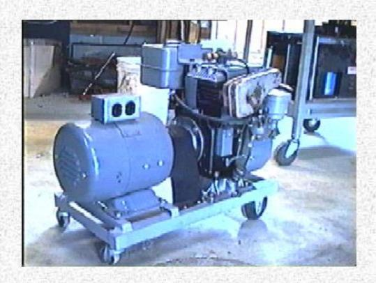
Model 1W532 1700 Watts 115V 60 Cycles 14 Amps 3600 RPM Generator No. 2M094
