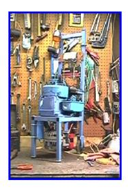
B&S/Chrysler Alternator12 VDC @ 50 A
