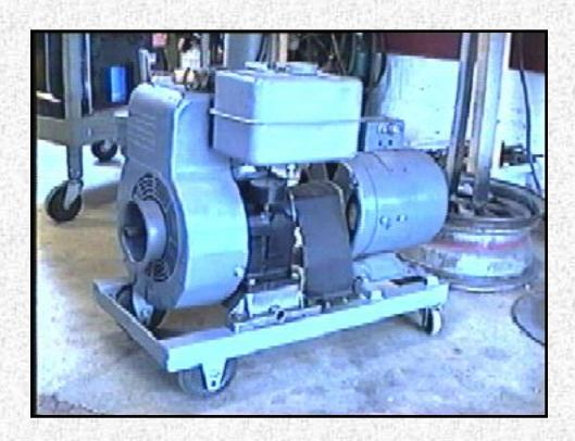
The AC jack on the generator is actually an electrical workbox that I welded to the old mounting plate. The previous box was smashed. There are two big electrical connections on the back of the plate. I thought that they were for battery charging, but upon a closer inspection of the label I found that the connections were for a STARTING battery! Apparently the generator acts as a starting motor when 12 volts is placed across these terminals. Yep, it really works!
