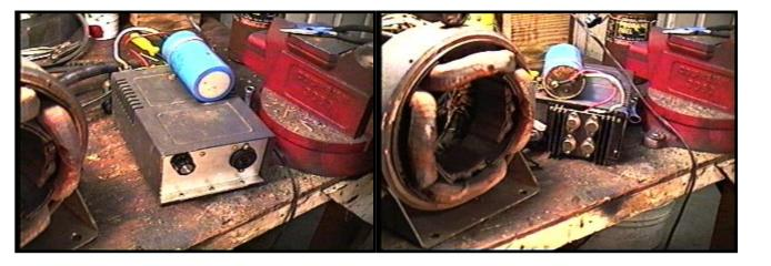
I have 4 pass transistors on the back of it heatsinked. The regulator has to power the 4 poles as electromagnets so it passes a lot of current. I think it is about 6 to 8 amps.
