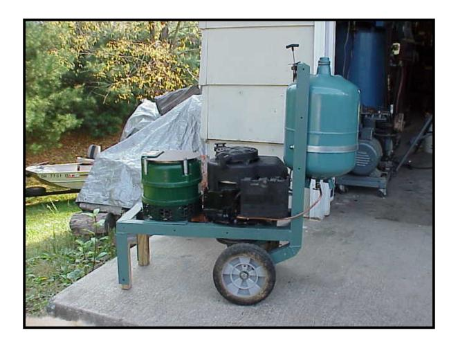
Finished product. Note that I finally found a use for that empty freon tank! It was a tank that held 30 lbs of R-134A. Now it holds about 3.6 gallons of gasoline, giving me at least 12 hours of run time.
