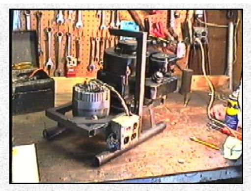
It is capable of 700 watts at 120 Volts AC or DC output. The AC frequency is about 250 to 400 hz, depending of engine speed. You may ask, "What can you power at that frequency?" Plenty! Lightbulbs don't care what frequency they operate at. Devices that are power-transformer operated, such as a radio, TV, VCR, etc. work very well on this frequency.
