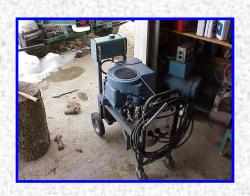
Here is a new welder/generator that I've just finished in February, 2000. It is a 100 ampere DC welder, powered by a B&S 8 hp gasoline engine. Click on it to go directly to this welder page.
