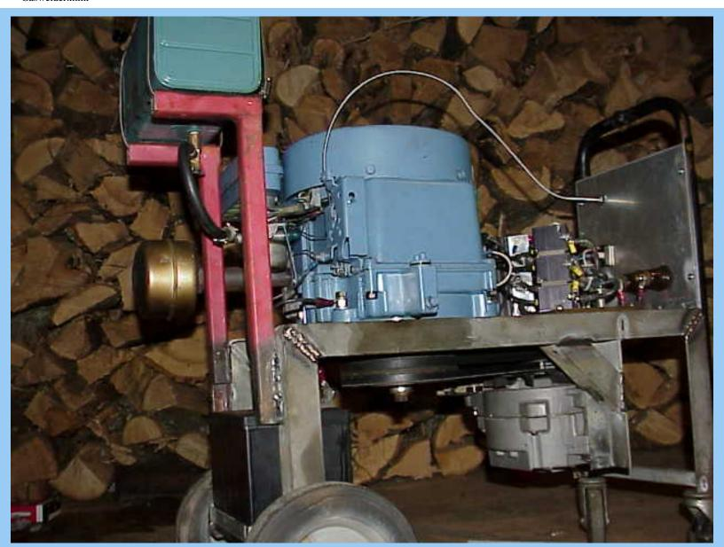
Another view of the left side. The exhaust pipe is either going to be shielded or moved from under the gas tank for saftey reasons.
