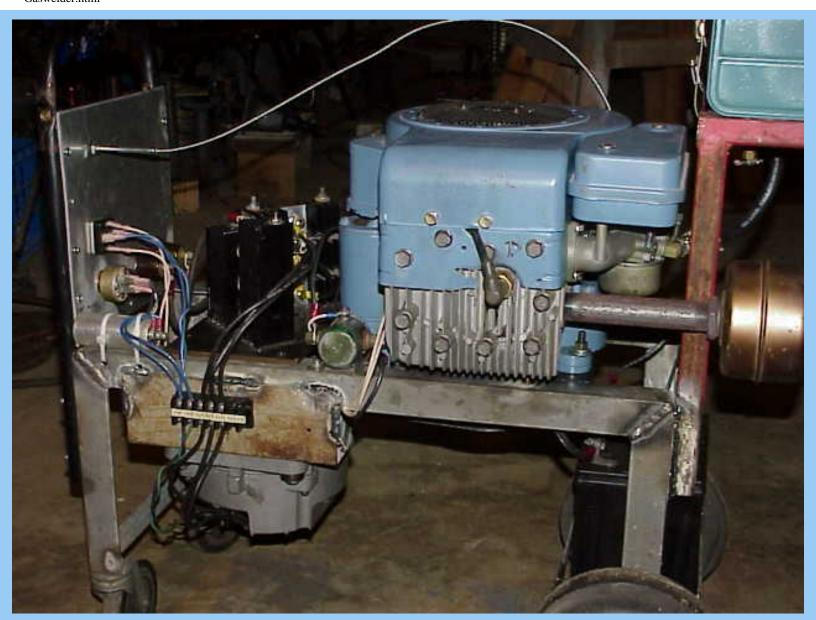
The terminal block above the alternator has, from left to right: Field power, negative and positive, then the three wires from the three phases from the alternator.
