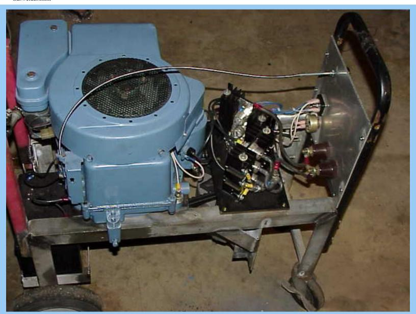
In this view the three phase diode bank with its black heat sinks can be readily seen between the engine and the front panel.
