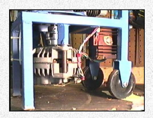
Side view of the alternator, voltage regulator and Lovejoy coupling.
