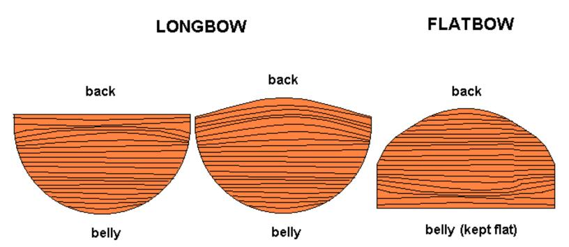
(the back remains flat, or slightly convex, following the natural line of the growth rings and the sides and belly slightly rounded into a "D" shape. Wood is shaved off with rasp, spokeshave, drawknife or scraper untill the appropriate tiller is maintained, all the time ensuring that the slope of the taper remains constant from handle to tip.)
