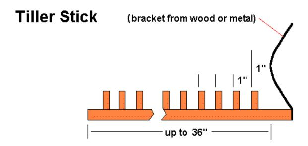
wooden dowel pins glued/or slots cut into base at 1" intervals from bracket.
