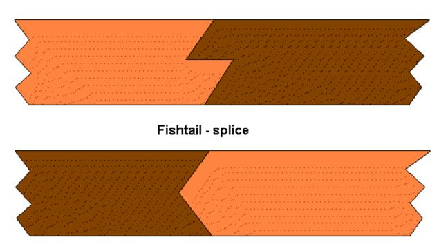
This can also be done if you are unable to find a single length of wood to make a complete stave. 2 half-lengths can be spliced using either of the above splices, such that the spliced section will be in the handle section of the bow and therefore covered by the handle wrapping etc.
