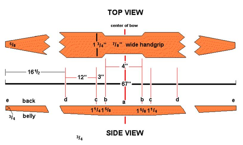
(NB, the bow is drawn to 67" length, designed for a 28" draw length. If your draw length is longer or shorter, alter the total length by 2" for every 1" draw length change (e.g. draw length of 26" gives a length of 63") Handle section (c-c) remains the same, the rest (c-e) should alter in proportion.)
