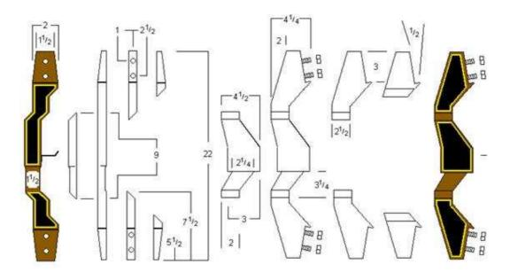
This construction is made up of 3/4" board lengths cut and glued together to achieve the same result as a solid carved piece.
