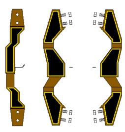
This construction is made up of 3/4" board lengths cut and glued together to achieve the same result as a solid carved piece.
