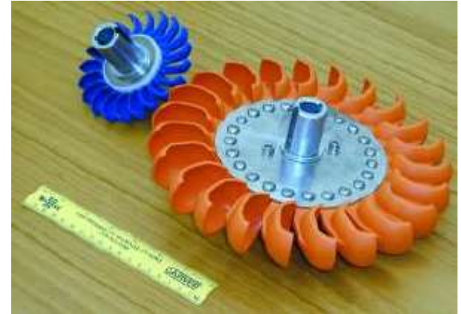
Find the runner diameter to match site head and rpm.
