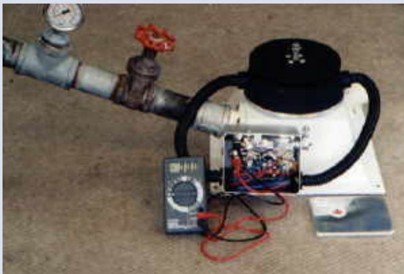
Stream Engine showing multi-meter used to measure output current.
