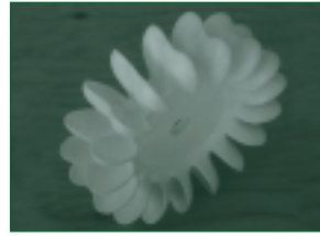
Polyurethane Pelton Wheel 10cm/4" pitch diameter
