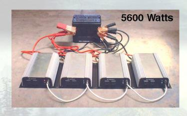
Each power inverter in the stackable modular array is rated at 1400 watts. You may put together as many as you wish for all the power you ever need!
