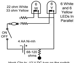
Hook Clip to -12 V DC turn on the switch and + Terminal to charge the 4 AA cells
