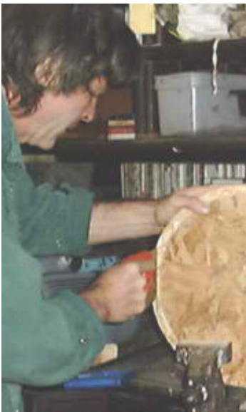
Sawing flat faces on the inner mould
