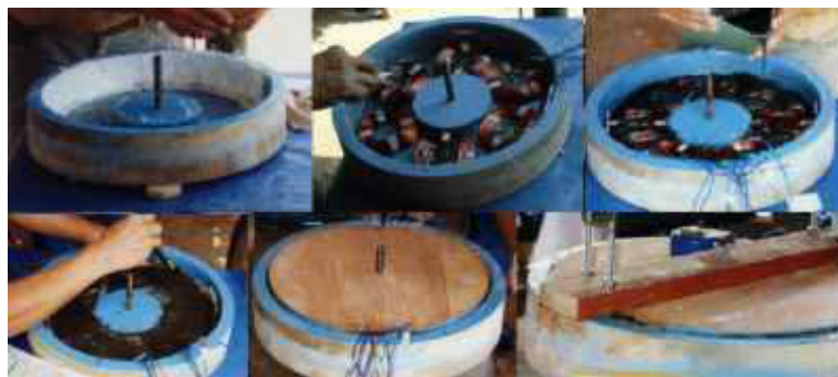
Six stages of the rotor casting procedure
