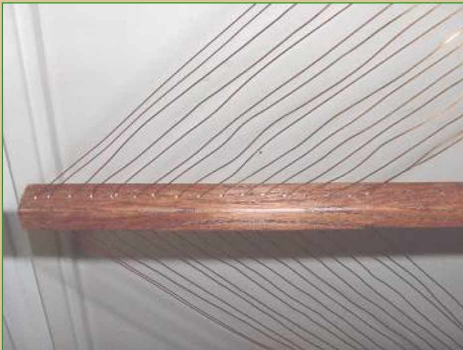
Left side arm showing 17 holes with wires.
