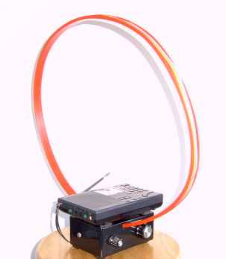
The portable loop in use, the portable radio is simply placed into the centre of the loop and the signals collected are inductively coupled to the internal ferrite rod antenna of the radio
