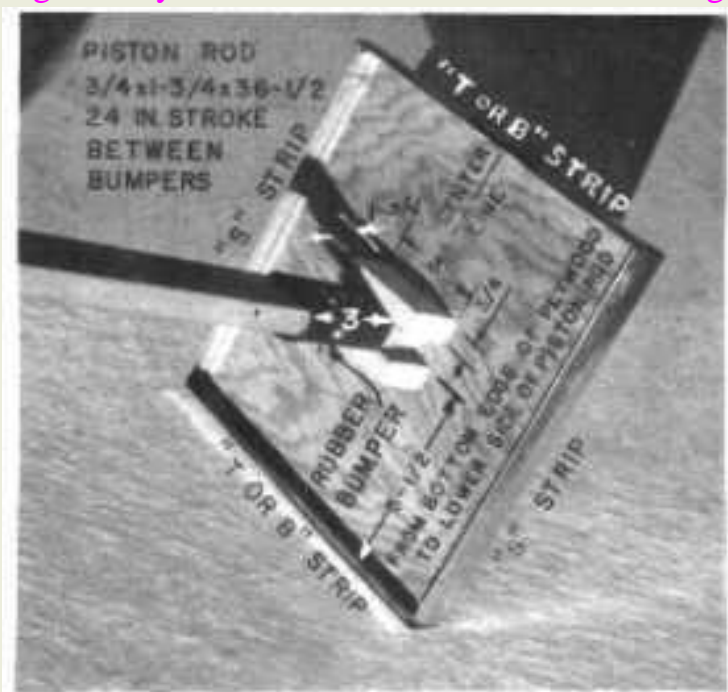
Fig. 14. Plywood Piston with Sheetmetal Sealing Strips Attached.
