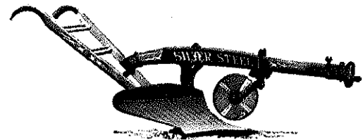
By the late nineteenth century, steel breaking plows were widely available. This steel plow has a wooden beam and a disk couler.
