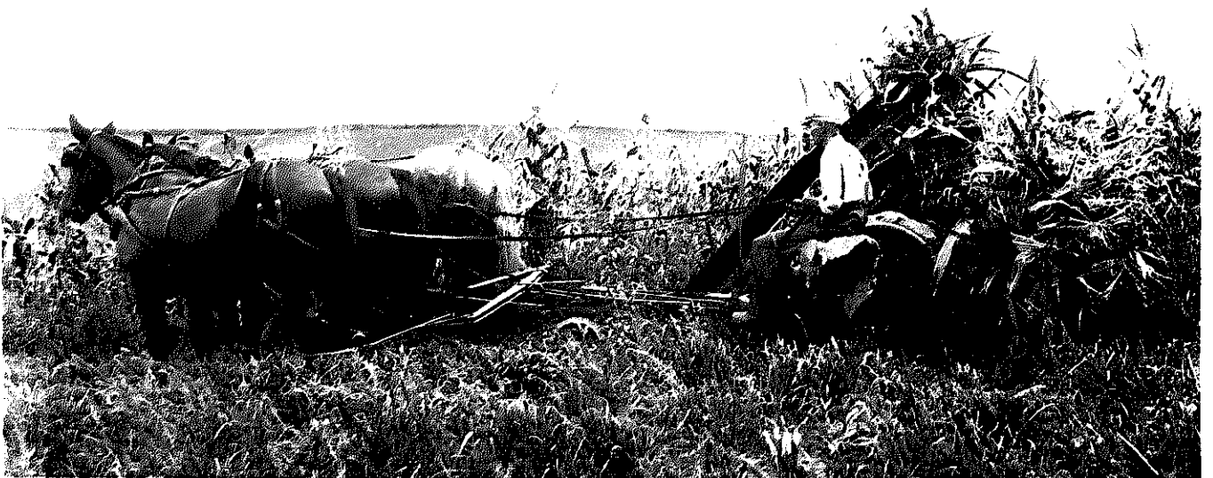
Below: By the mid-1880s, the mechanical problems of the corn binder had been eliminated. Generally, three horses were required for draft. (National Archives.)
