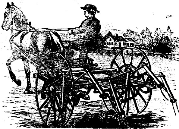
In 1882, the Bullard Hay Tedder was built by the Richardson Manufacturing Company of Worcester, Massachusetts. By the 1890s, steel had replaced wood for tedder frames. The Quail All Steel Tedder, manufactured by the Ohio Rake Company of Dayton, Ohio, is a notable example.
