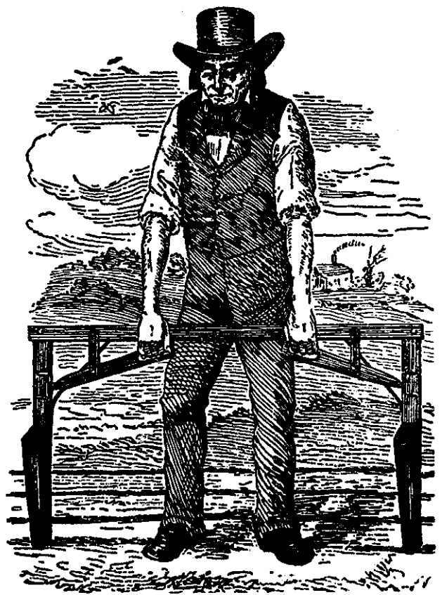
The Randall and Jones Double Hand Planter enabled a farmer to seed his crop in evenly spaced rows for easier cultivation. (Smithsonian Institution.)
