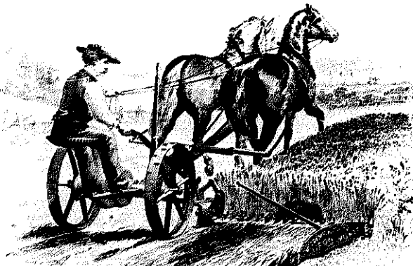
In 1884, the McCormick Harvesting Machine Company offered this mower for sale. Note that the gears at the center of the axle have been covered to keep out the dust.
