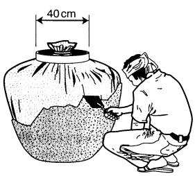
4. Place a metal ring on top of the jar as a mould for the opening. Place the first layer of mortar onto the sacking to a thickness of 0.5 cm.
