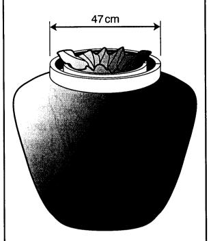
5. Add a second layer of mortar to give a total thickness of 1cm. Check thickness of mortar by pushing in a nail. Form an opening at the top with a second metal ring.
