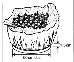
2. Place sack on a pre-cast mortar bottom plate, 60 cm dia. × 1.5 cm thick. Fill sack with sand. Ensure bottom plate sticks out from under the sacking.
