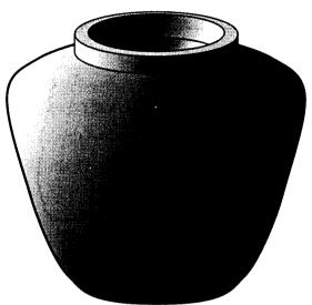
6. Remove the sand, sacking and rings two days after plastering. Repair any defects with mortar. Paint the inside with cement slurry. Cure for two weeks.
